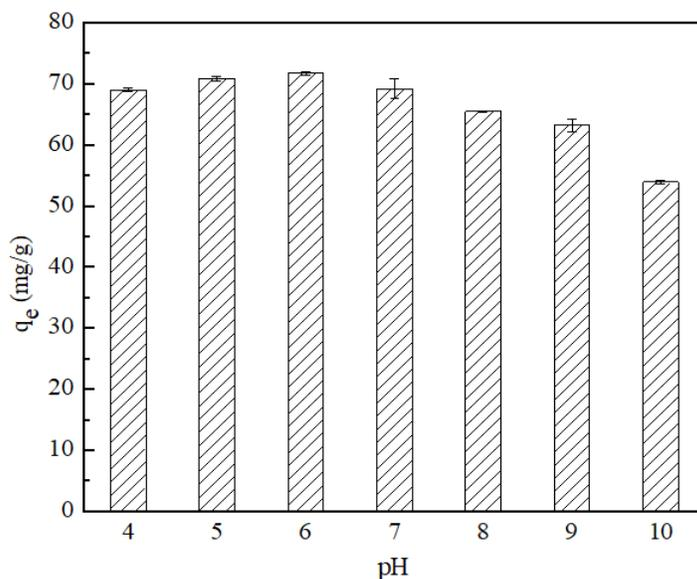
**Figure 3** The effects of solution pH on the removal of As(V) by AZBO. (Experimental conditions: initial As(V) = 7.5 mg/L, pH = 4.0~10.0, adsorbents dosage = 0.3 g/L, ion strength = 0.01 mM NaNO<sub>3</sub>)
