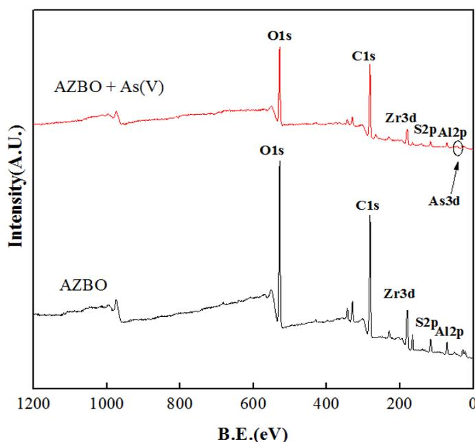
**Figure 6** The XPS all-scan spectra of AZBO before and after As(V) adsorption. (Experimental conditions: initial As(V) = 7.5 mg/L, pH = 7.0, adsorbents dosage = 0.3 g/L, ion strength = 0.01 mM NaNO<sub>3</sub>)
