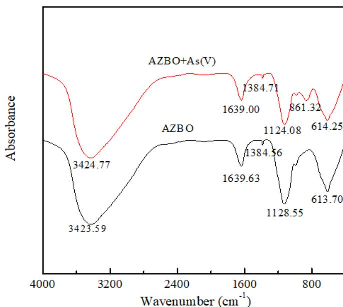
**Figure 5** The FTIR spectra of AZBO before and after As(V) adsorption. (Experimental conditions: initial As(V) = 7.5 mg/L, pH = 7.0, adsorbents dosage = 0.3 g/L, ion strength = 0.01 mM NaNO<sub>3</sub>)
