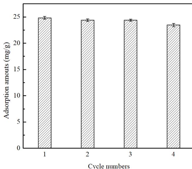
**Figure 8** The performance of AZBO for the adsorption of As(V) in four consecutive adsorption-desorption cycles. (Experimental conditions: initial As(V) = 7.5 mg/L, pH = 7.0, adsorbents dosage = 0.3 g/L, NaOH = 0.1 mM, ion strength = 0.01 mM NaNO<sub>3</sub>)
