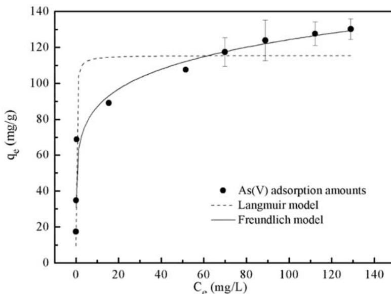
**Figure 2** The isotherm curve of As(V) adsorption onto AZBO. Symbols indicate experimental data; solid lines represent the Freundlich model; dash lines refer to the Langmuir model. (Experimental conditions: initial As(V) = 3.75~120 mg/L, pH = 7.0, adsorbents dosage = 0.3 g/L, ion strength = 0.01 mM NaNO<sub>3</sub>)
