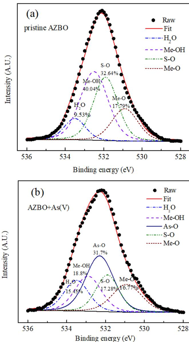
**Figure 7** The O1s XPS spectra of AZBO before and after As(V) adsorption. (Experimental conditions: initial As(V) = 7.5 mg/L, pH = 7.0, adsorbents dosage = 0.3 g/L, ion strength = 0.01 mM NaNO<sub>3</sub>)
