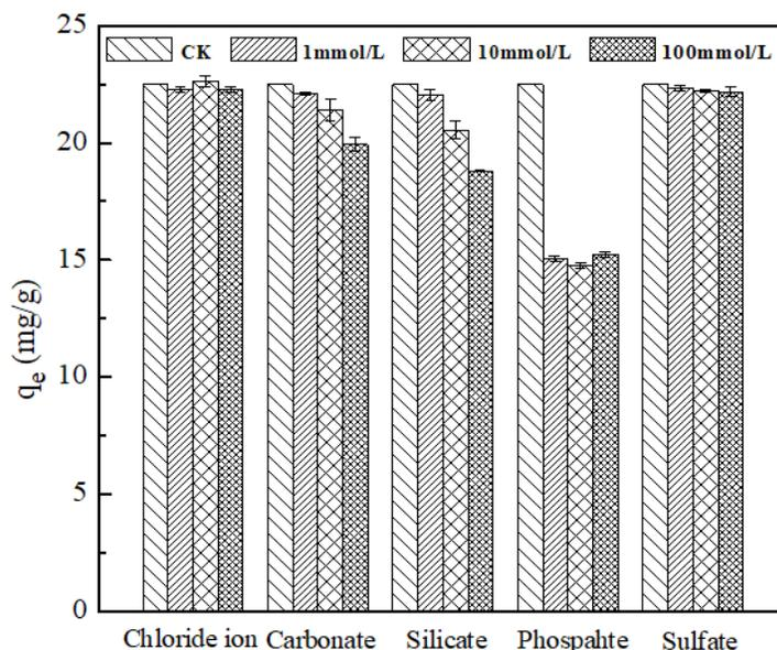
**Figure 4** The effects of coexisting anions on the removal of As(V) by AZBO. (Experimental conditions: initial As(V) = 7.5 mg/L, pH = 7.0, adsorbents dosage = 0.3 g/L, ion strength = 0.01 mM NaNO<sub>3</sub>)
