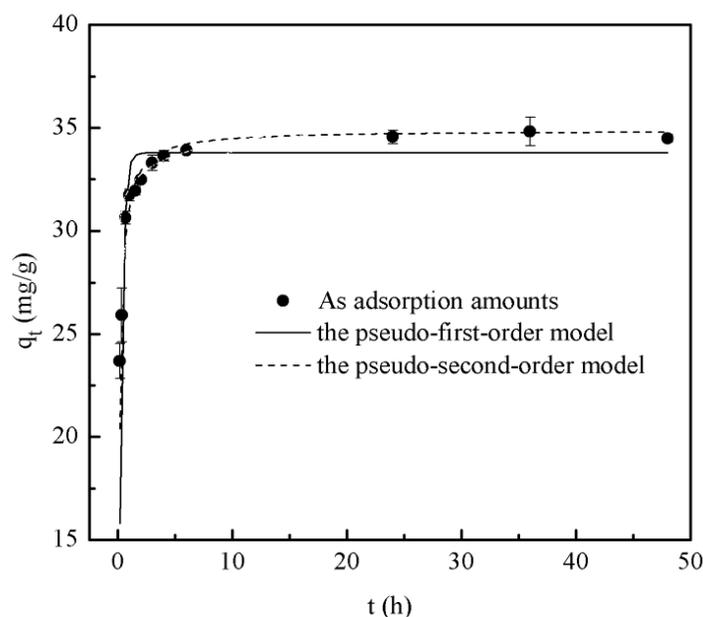
**Figure 1** The kinetic curve of As(V) adsorption onto AZBO. Symbols indicate experimental data; solid lines represent the pseudo-first-order model; dash lines refer to the pseudo-second-order model. (Experimental conditions: initial As(V) = 7.5 mg/L, pH = 7.0, adsorbents dosage = 0.3 g/L, ion strength = 0.01 mM NaNO<sub>3</sub>)
