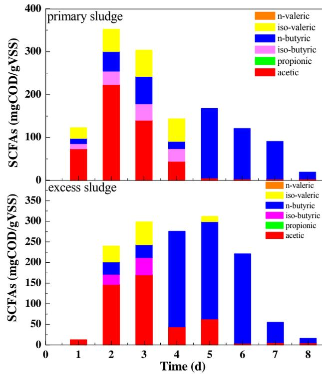
Figure 3 SCFAs components in sludge fermentation
