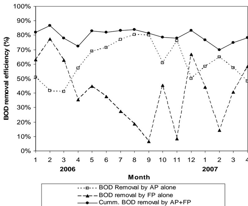
Figure 11 Performance of Anaerobic & Facultative ponds for the removal of BOD
