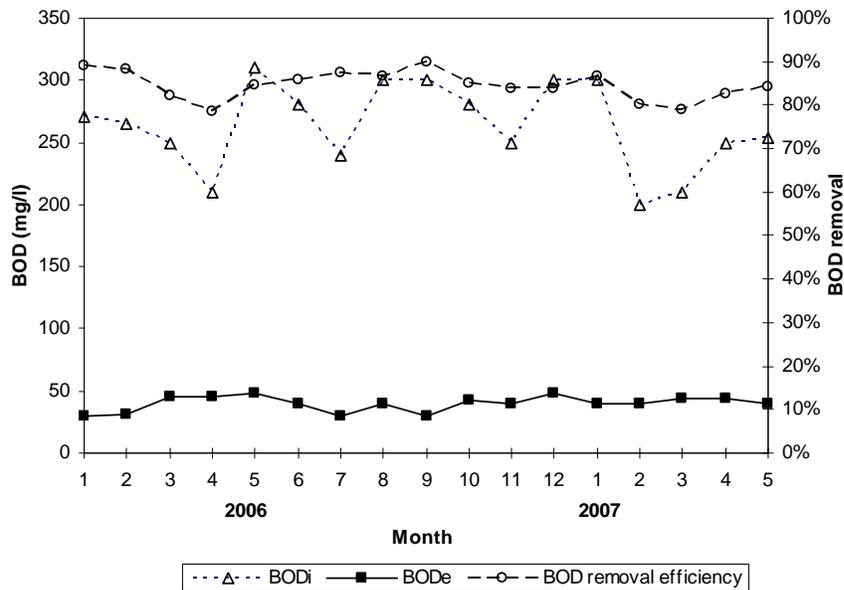
Figure 9 BOD variation of the influent and the effluent & the BOD removal efficiency of STP
