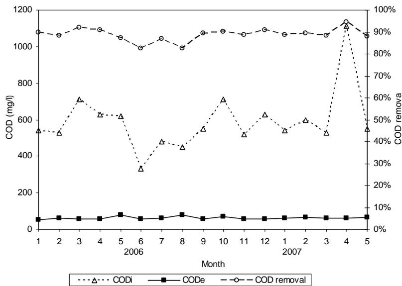
Figure 10 Variation of influent and effluent COD and removal efficiency
