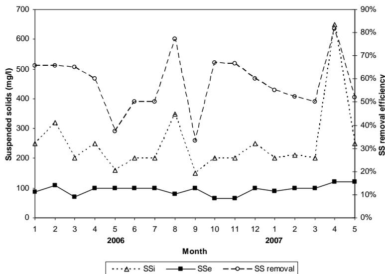
**Figure 8** SS variation of the raw sewage and the effluent & the SS removal efficiency of STP
