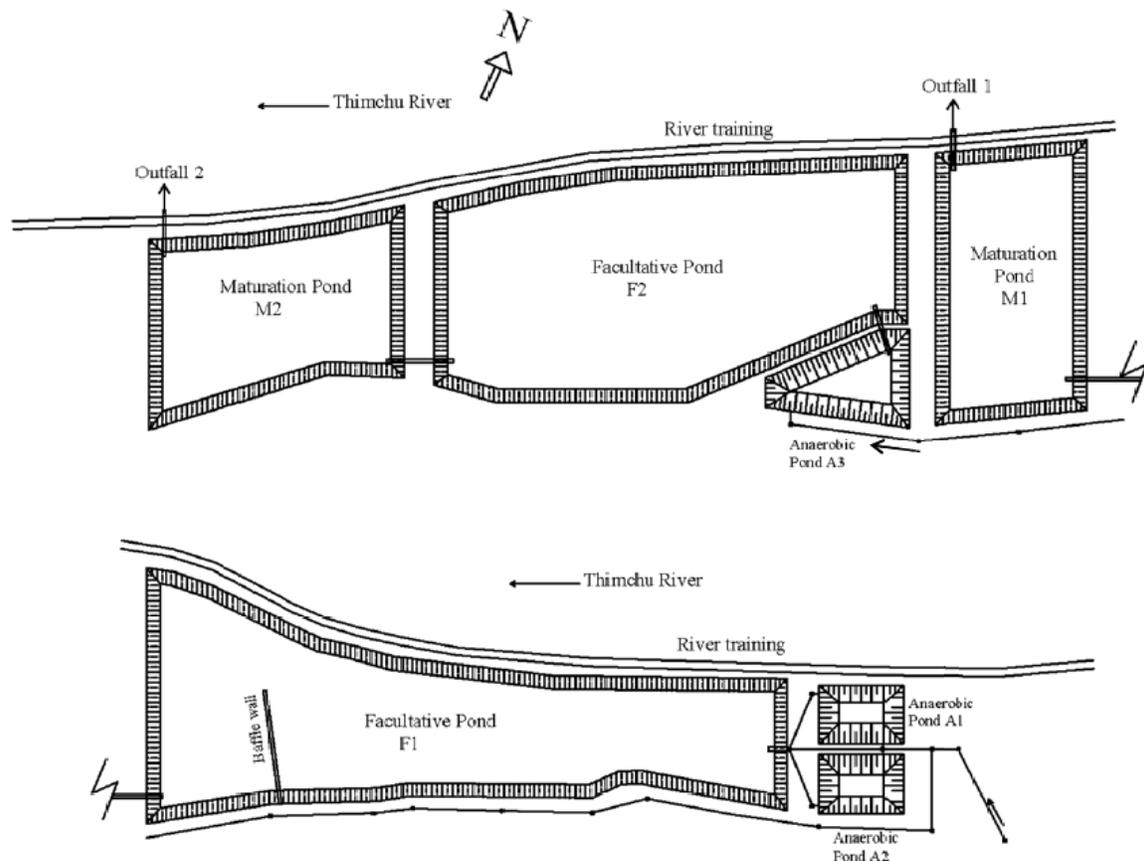
**Figure 3** Schematic lay out plan of Thimphu waste stabilization ponds
