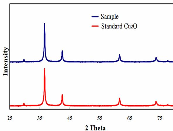
**Figure 2** XRD patterns of standard  $\text{Cu}_2\text{O}$  and sample
