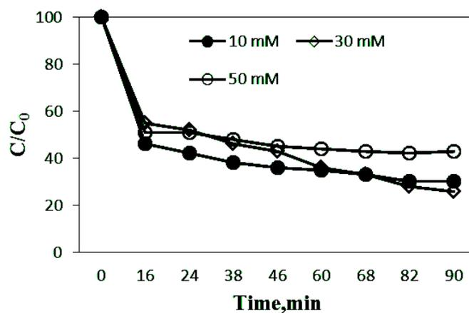
**Figure 6** Residue of BPA under UV365 nm irradiation and various H<sub>2</sub>O<sub>2</sub> (C<sub>0</sub>=10 mg/L, T=25±2°C, flowrate=2.8 cm<sup>3</sup>/min, light=2.79 mW/cm<sup>2</sup>)
