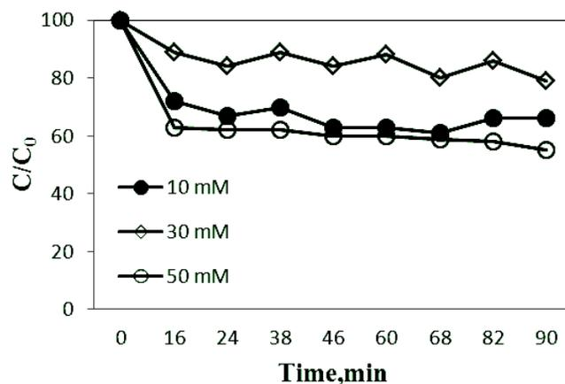
**Figure 5** Residue of BPA reacting with various H<sub>2</sub>O<sub>2</sub> (C<sub>0</sub>=10 mg/L, T=25±2°C, flowrate=2.8 cm<sup>3</sup>/min)
