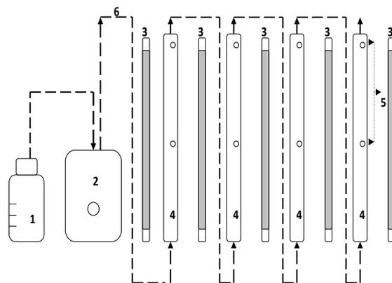
**Figure 1** Photocatalytic system (1.tank for BPA solution 2.pump 3.UV light 4.reactional column system 5.sampling part 6. pipeline)
