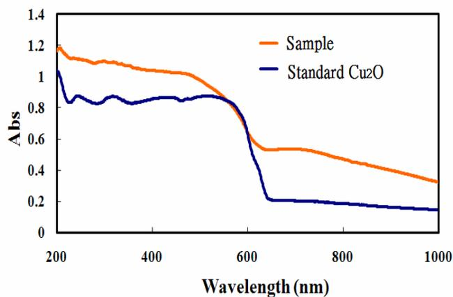
**Figure 3** UV-vis spectrum of standard  $\text{Cu}_2\text{O}$  and sample
