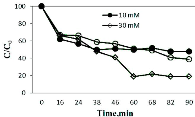
**Figure 7** Residue of BPA using a Fenton-like process at various H<sub>2</sub>O<sub>2</sub> (C<sub>0</sub>=10 mg/L, T=25±2°C, flowrate=2.8 cm<sup>3</sup>/min, Cu<sub>2</sub>O=0.112 g)
