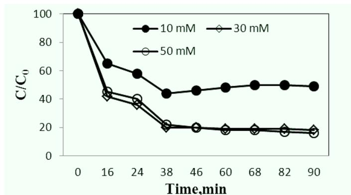
**Figure 8** Residue of BPA using a photo Fenton-like process at various  $H_2O_2$  ( $C_0=10$  mg/L,  $T=25\pm 2^\circ C$ , flowrate= $2.8$  cm<sup>3</sup>/min, light= $2.79$  mW/cm<sup>2</sup>,  $Cu_2O=0.112$  g)
