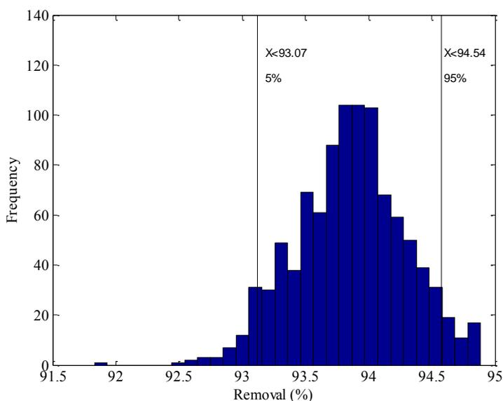
**Figure 5** Simulated PDF of TP removal (%) from influent to effluent at WRAMS
