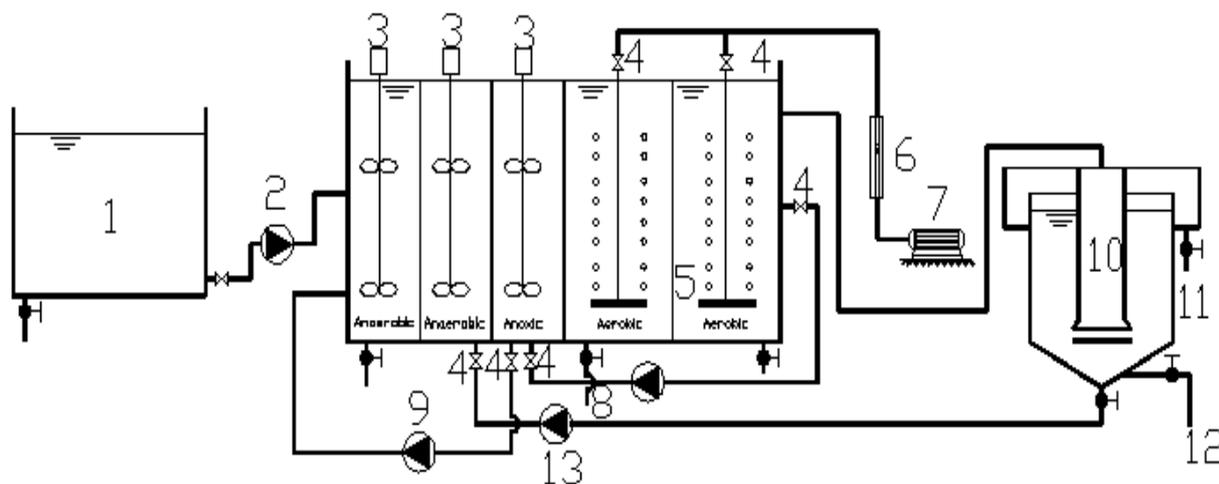
**Figure 1** Schematic diagram of lab-scale anaerobic/anoxic/oxic EBPR reactor. 1. Influent tank; 2. feed pump; 3. mechanical mixer; 4. check valve; 5. diffuser; 6. airflow meter; 7. air compressor; 8. return nitrifying liquor pump; 9. recycling mixture liquor pump; 10. secondary clarifier; 11. effluent; 12. waste sludge; and 13. return sludge pump
