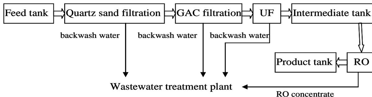
**Figure 1** The schematic of electroplating wastewater treatment process
