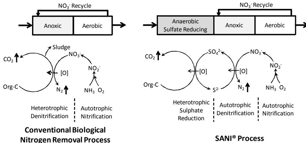
**Figure 2** Conventional BNR process, the SANI<sup>®</sup> process and the S-C-N cycle theory
