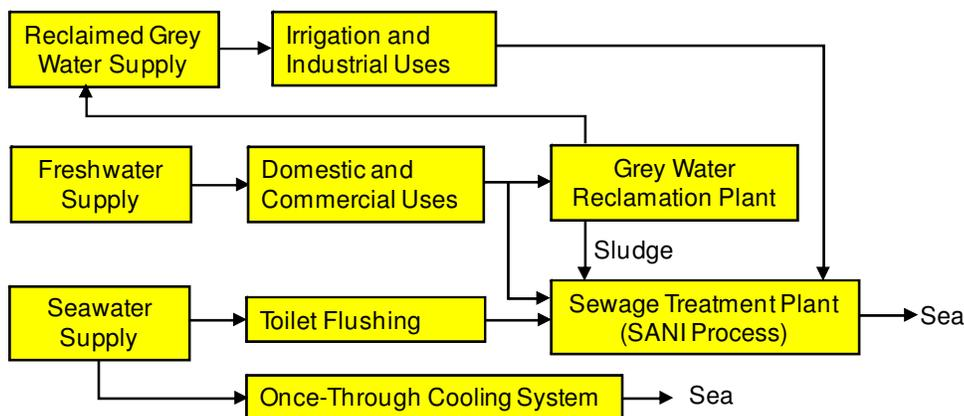
**Figure 1** Conceptual diagram of the TWS system
